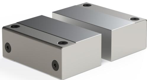
Our Anti-Lift Jaws use a cleat and angled soft jaw to pull the jaw in and down when torque is applied to the lead screw. This design decreases jaw lift and jaw deflection commonly seen in self-centering vises.
