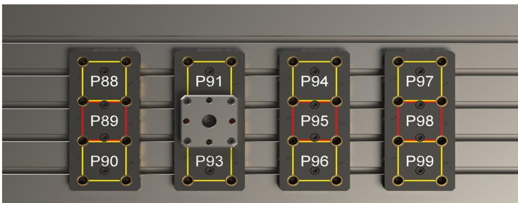
1. Starting with an empty machine table, install 5th Axis 3613S plates for your specific table. Thread bolts into t-nuts, but do not torque bolts.
