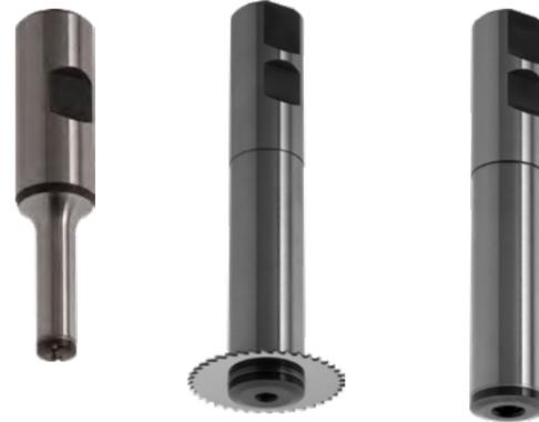
For the precise use of your saw blade holder, please pay attention to the correct insertion of the washer (see picture below). When choosing your cutting data, e.g. cutting speed and the feed rate, please take into account that your saw blade is only held by surface pressure. Too high cutting data or a dull saw blade can lead to hooking or stopping of the saw blade which can result in damages at your workpiece, saw blade, saw blade holder or even at your machine.
