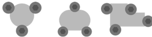
**Safely fixed:** the clamping screws are added from above. They clamp the workpiece powerfully and securely. A soft exchangeable brass ring avoids damages or scratches at the workpiece.
