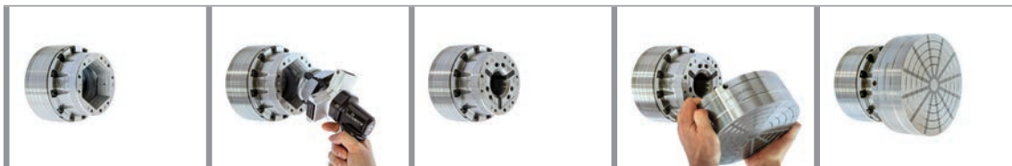
Remove clamping head
